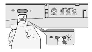
Be sure to insert the Memory Stick in the correct direction. If the Memory Stick is forced in the wrong way, it may become damaged.
